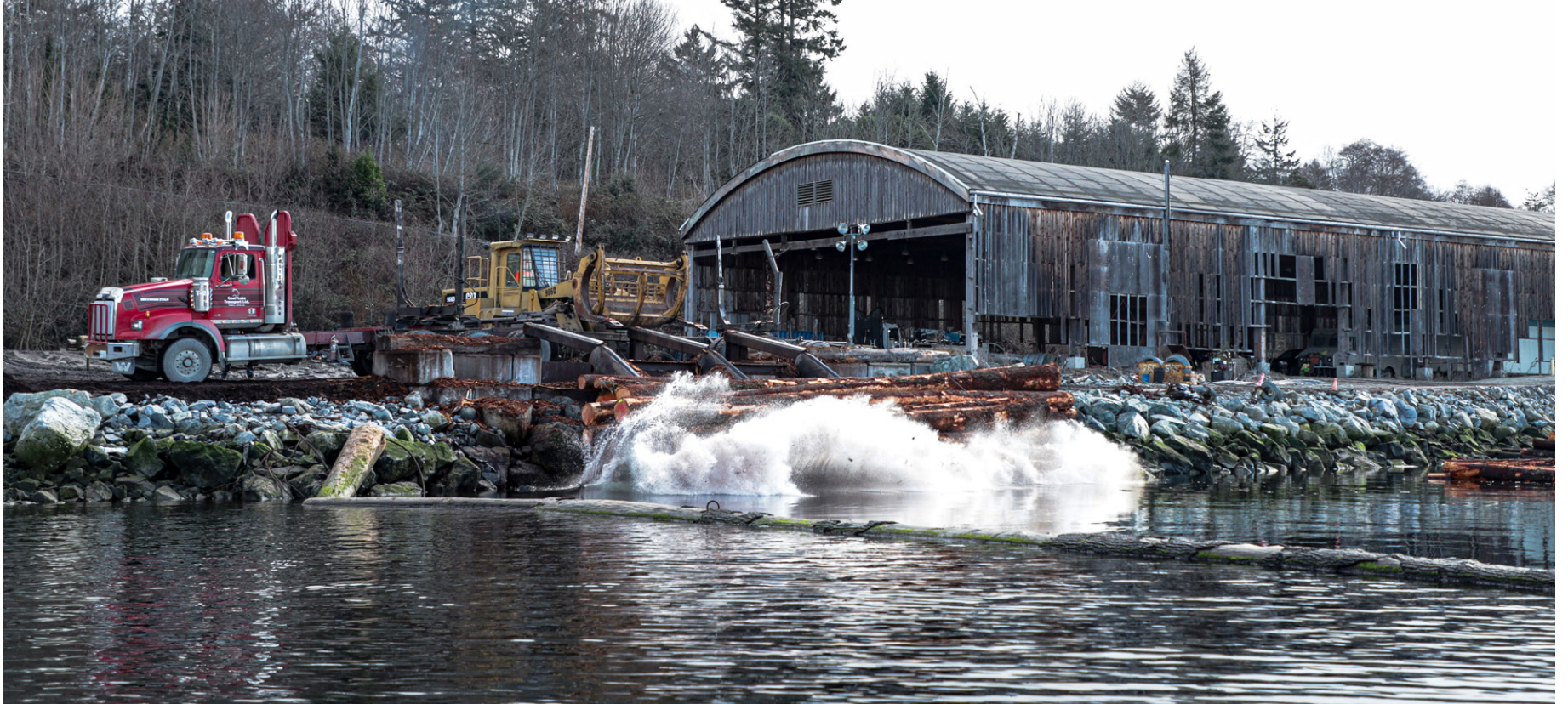
MAKING A SPLASH: Wayne Noble works the yellow skidder, pushing the logs off the truck into the water. This log dump site by the Hulks beach has been recently acquired by Tla'amin Nation's Thichum Forest Products. Photo by Abby Francis
