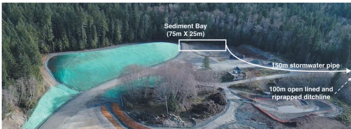
Above is a drawing of a proposed $850,000 engineered solution that would have required cutting down a half hectare of trees to make a sediment bay. Instead, the December 2020 image below shows the system built, keeping the trees and using the forest to help disperse stormwater runoff. This method saved $700,000.
