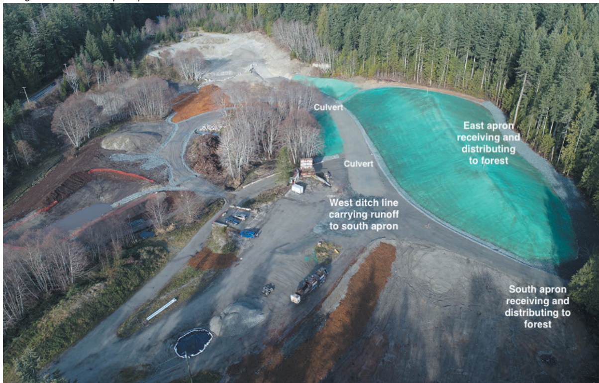
Above is a drawing of a proposed $850,000 engineered solution that would have required cutting down a half hectare of trees to make a sediment bay. Instead, the December 2020 image below shows the system built, keeping the trees and using the forest to help disperse stormwater runoff. This method saved $700,000.
