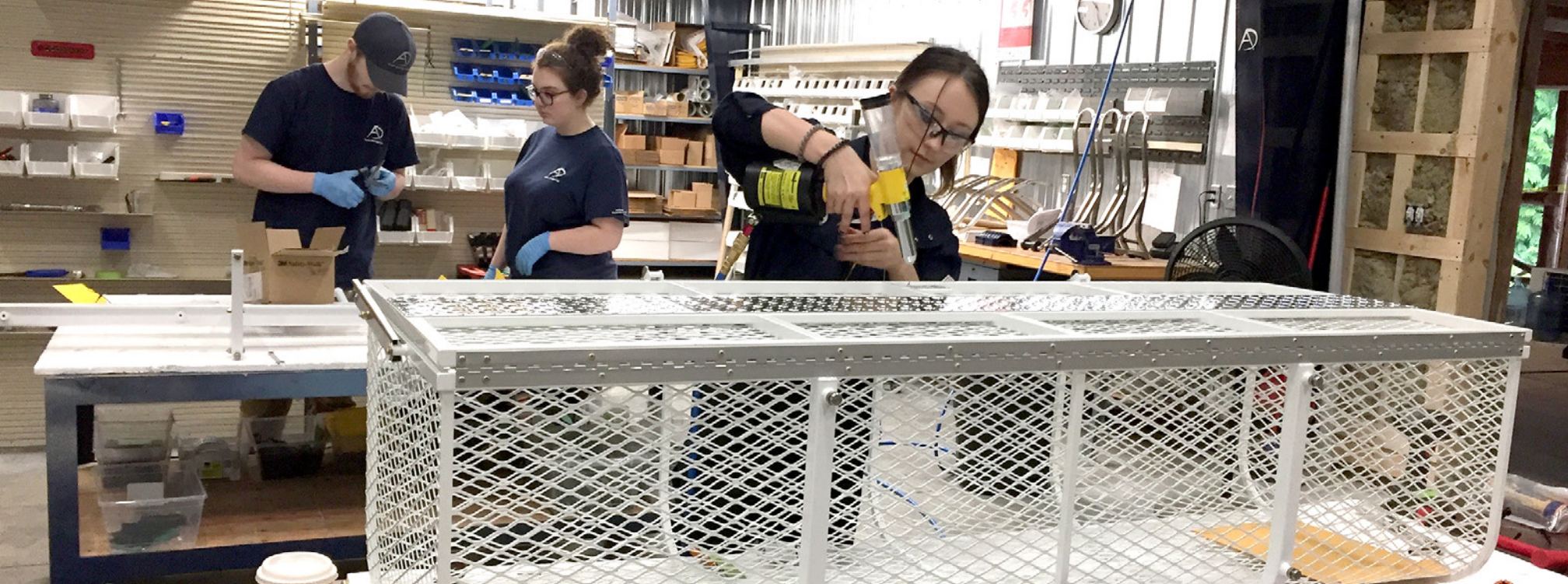
MAKING IT: Mira Bolton Hicks rivets a data plate on a cargo basket. In the background, Nick Rekve and student Grace Desilets package up some parts for shipment.
