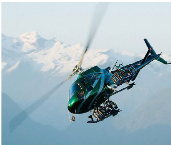
PRECIOUS CARGO: Aero Design bicycle racks on an Airbus AS350. The racks belong to Nimmo Bay Resort and the helicopter is operated by West Coast Helicopters. photo courtesy of Nimmo Bay Resort
